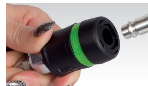
Safety Quick Coupling: one pull and the compressed air is dumped. One push and the adaptor is safely disconnected
