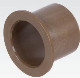
Plain bearing flange bush from high sophisticated thermoplastic. Very low friction. Specially suited for dry-running and for use under water and at high temperatures. Colour: brown.
