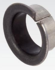
Plain bearing flange bush from steel sheet with multi-porous bronze layer and sliding surface from PTFE-lead-compound. Specially suited for lubrication-free running, for high loads, extrem temperatures.
