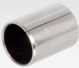
Plain bearing bush from steel sheet with multi-porous bronze layer and sliding surface from PTFE-lead-compound. Specially suited for lubrication-free running, for high loads, extrem temperatures.
