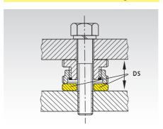
The Spacer **DS** is used to bridge gaps between the levelling adjuster and the bearing surface when the adjustment travel  $\Delta h$  is insufficient.
