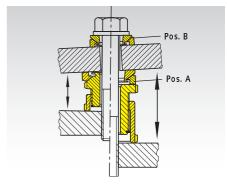
Like the ball head precision adjusters KAE the ball shim **KAS** (Pos. A) facilitates adjustment of non-parallel surfaces with an angle of inclination of up to 4°. If the angle of inclination  $\alpha > 1^\circ$ , the use of an additional ball shim (Pos. B) is recommended to assure a stable support of the bolt head.
