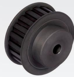
**Material:** Up to a Teeth Number of 48 phosphated steel, from a Teeth Number of 50 grey cast iron GG20. Pre-bored.
