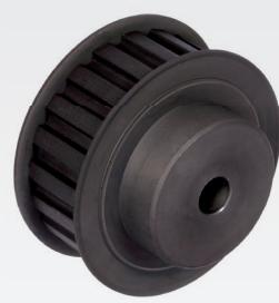
**Material:** Up to a Teeth Number of 40 phosphated steel, from a Teeth Number of 44 grey cast iron GG20. Pre-bored.
